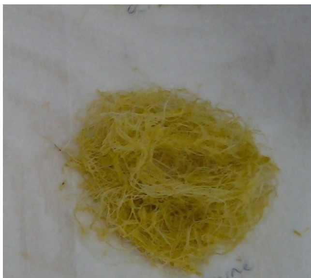
Figure 1. Photography image of the extracted corn husk fibers.
